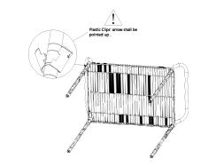
4 Slide down the wire shelf(A) down onto the plastic clips and set the shelf upright.
