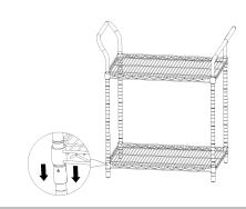
6 Slide the bumper(F)into the bottom of each pole,then screw the Rubber Casters (D) into the bottom of each Pole(B) in a clockwise direction and fasten it by wrench.
