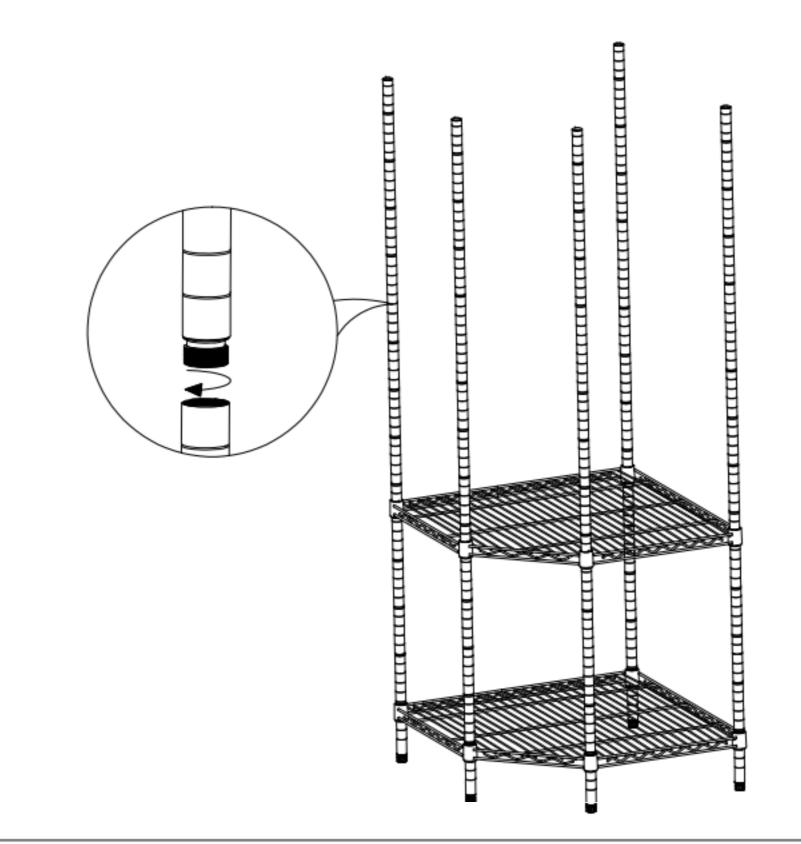
Refer to Step ①,② to snap plastic clips onto the same grooves of each pole for other two pieces wire shelves as the photo. Then assemble other two pieces wire shelves. Pushing firmly down on every wire shelf at corners by rubber mallet to ensure all the shelves are in a place over the plastic clips. Now the four tiers pentagon wire shelving
