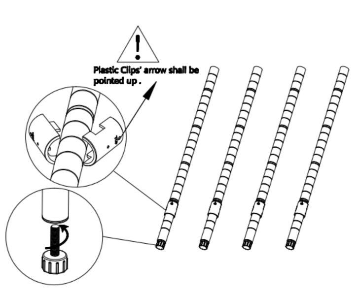
Please make sure that you have the Wire Shelf (A) correct way up. Hold the shelf on its side and slide it from the top of each lower pole down onto the plastic clips until there is snug fit.
