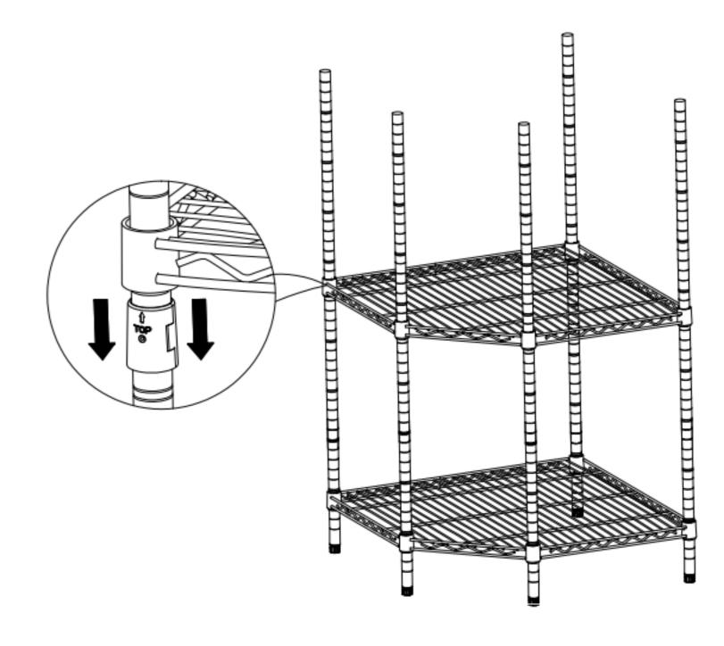
Screw Upper Poles (D) into lower poles by connectors which are already assembled on the upper poles.
