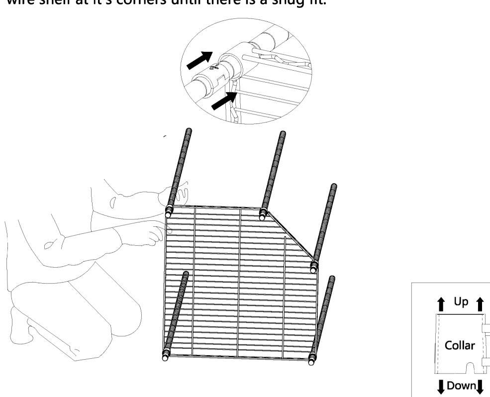
Set the wire shelf upright.Repeat step ①, ② to snap the plastic clips on the same groove of each pole at your next desired position and assemble the third wire shelf
