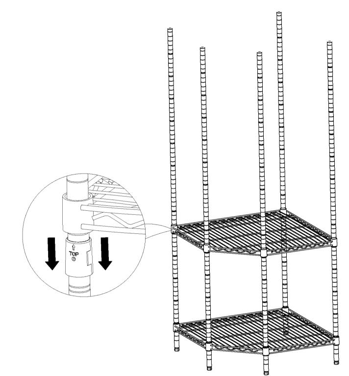
5 Snap plastic clips(D) into the top of each pole. Then Slide down the last shelf from top down onto the plastic clips.
