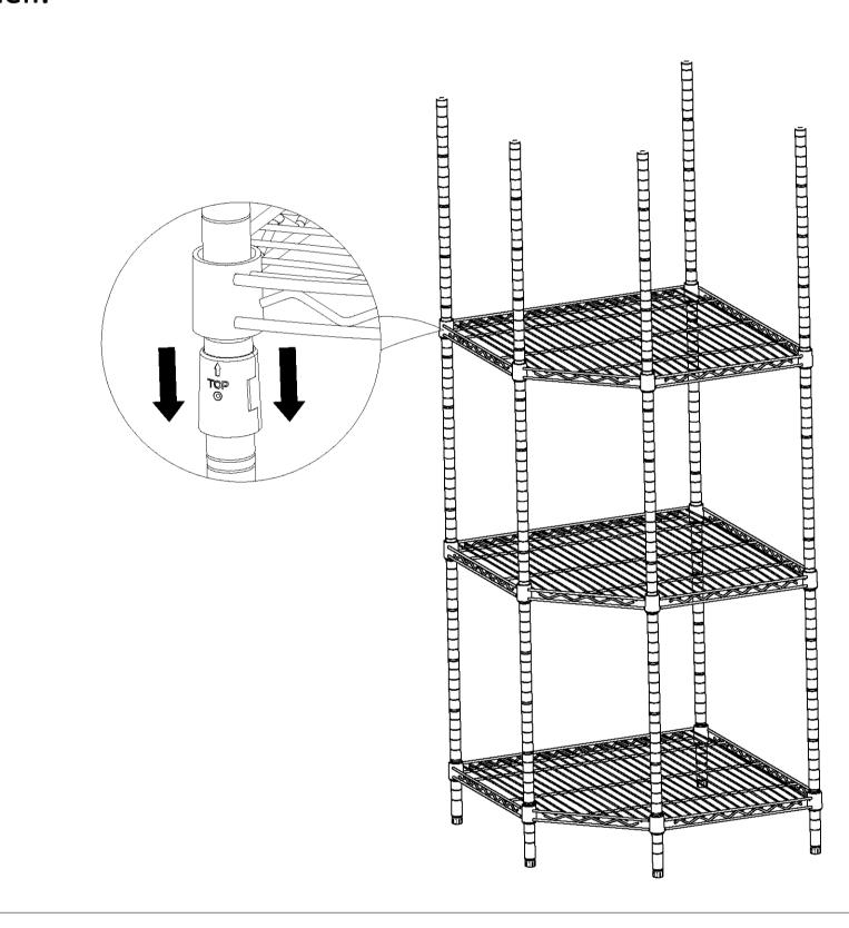
Once all the wire shelves have been installed, pushing firmly down on every shelf at corners by rubber mallet to ensure that the shelf in a place over the plastic clips. And screw the leveling feet in or out to attain proper leveling.
