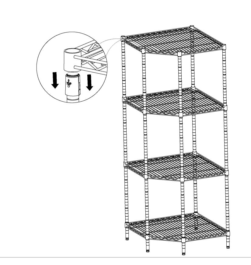
Please make sure that you have the Wire Shelf(A) the correct way up, hold the wire shelf on it's side and slide the top of four poles through the bottom of the wire shelf at it's corners until there is a snug fit.
