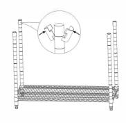
2 Hold the Wire Shelf (B) on its side and slide it from the top of each pole down onto the plastic clips until there is snug fit.
