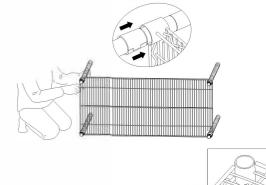
Put the Stainless Steel Plate (A) down onto the top of the rack until all plastic clips are well inserted the four collars welded under the stainless steel plate. Push firmly down on the shelf at its corner by rubber mallet to ensure the shelf in a place over plastic clips.
