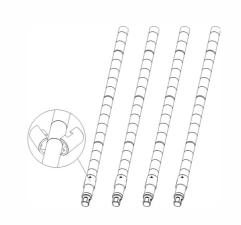
Set the rack upright. Refer to Step ① to snap one pair of plastic clips on the top of each pole.
