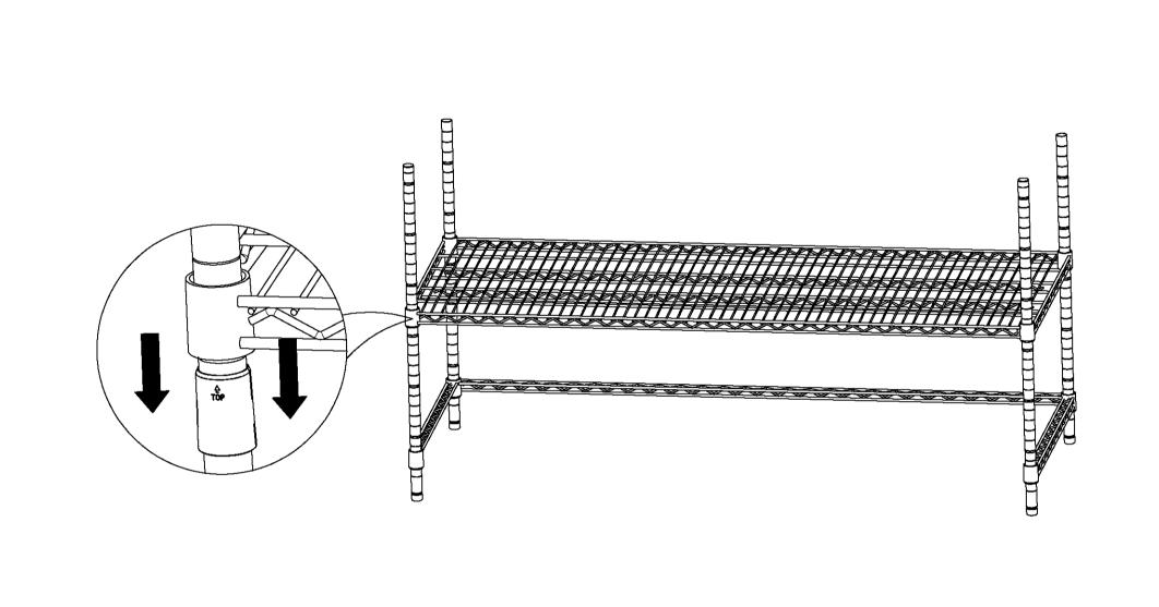
Screw Upper Poles (F) into lower poles(E) by connectors which are already assembled on the upper poles.
