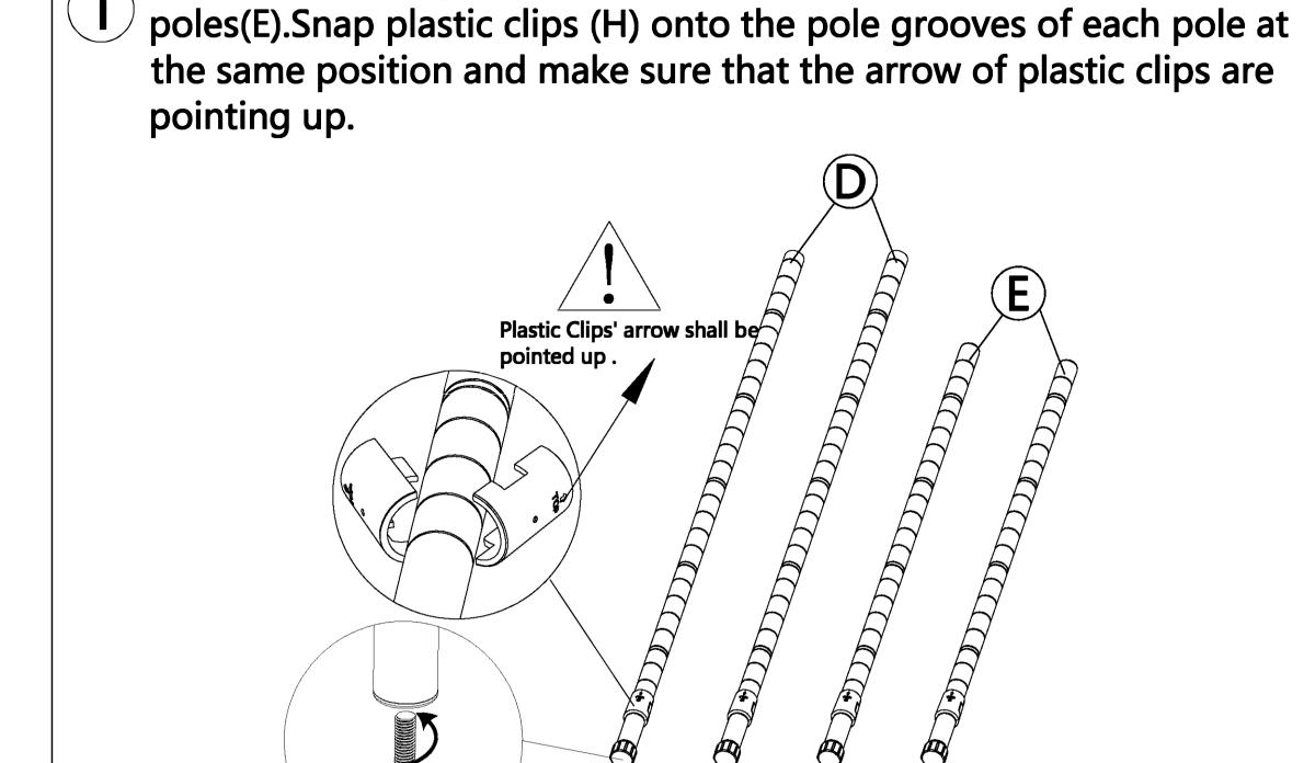
Screw the leveling feet(I) into the bottom of front pole(D) and Lower
