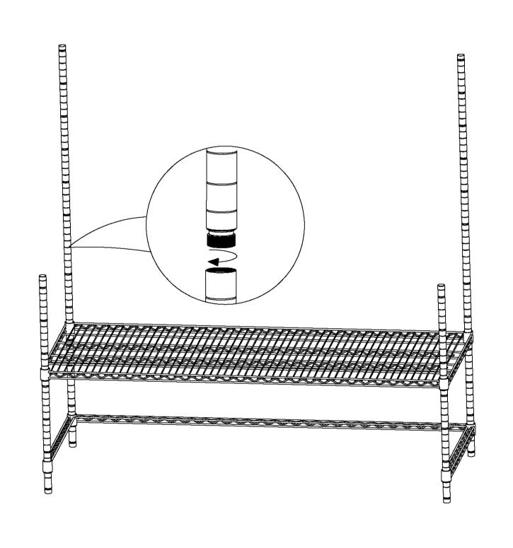
Snap plastic clips(H) into the top of front pole and lower pole of the same height. Then Slide down the second shelf from top down onto the plastic clips. Snap plastic clips(H) into the top of upper pole and slide down the semi-round wire shelf onto the plastic clips.
