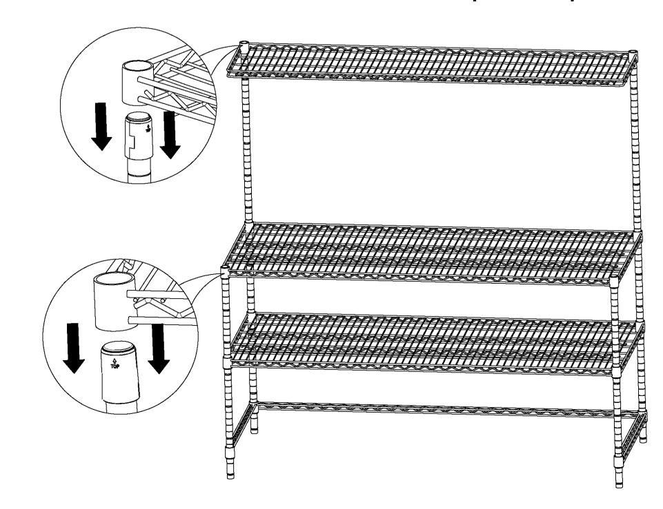
Once all the wire shelves have been installed, pushing firmly down on every shelf at corners by rubber mallet to ensure that the shelf in a place over the plastic clips.Put the PP mat(G) on the second wire shelf,then you finish the Installation.
