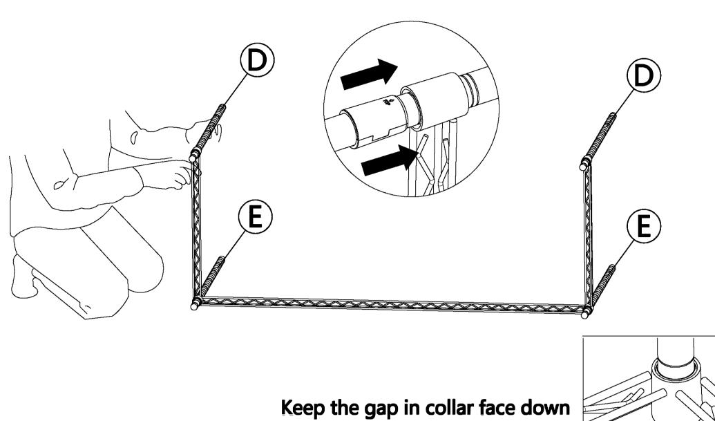
3 Set the wire shelf upright.Repeat step ①, ② to snap the plastic clips on the same groove of each pole at your next desired position and assemble wire shelf(A).
